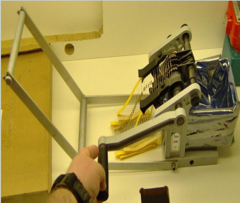
Manual cut and bend tool for axials on tape.
