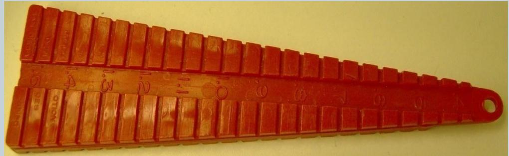
Hand-held resistor lead bending tool.
