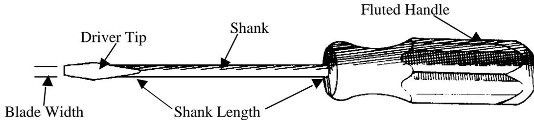
**Handles** - hardwood or plastic - may have a rubber grip for electrical protection, positive gripping, and comfort or it may have large flutes for improved gripping.
