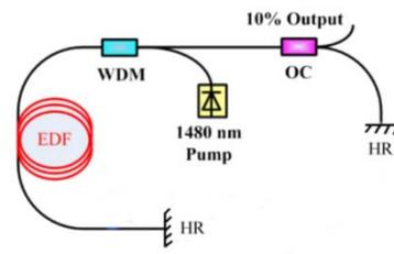
Note how the OC is different in this case – with a fiber laser it is frequently a coupler (and often measured in dB's ... 3dB=0.5, 10dB=0.1, etc).
