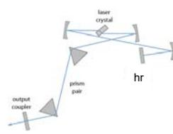
Assuming the OC is 2% transmitting, all other mirrors are 99% reflecting, the crystal is 1cm in length (and has essentially zero attenuation), and each prism absorbs 5% per pass due to absorption of the glass ...
