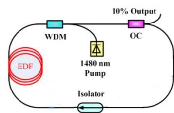
The isolator ensures lasing occurs in only one direction and can be considered lossless for this particular example.
