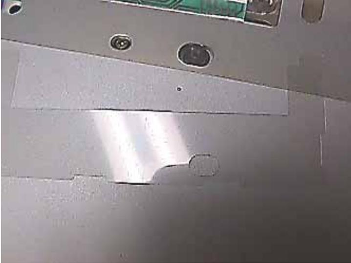
Before the PCB can be attached to the back plate, this thin plastic insulator must be aligned over the back plate to prevent the possibility of any exposed traces on the PCB from shorting out on the back plate when the keyboard is assembled. This film has several holes punched into it which only line up one way with holes in the mold and backplate, so locating the correct placement should be relatively easy.
