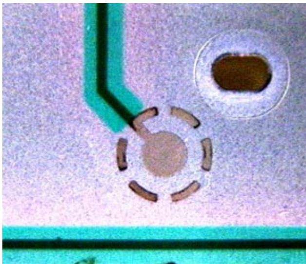
On the left, again, the enhanced photograph showing the damage to the keypad caused by the acid(s) found in many soda beverages. On the
