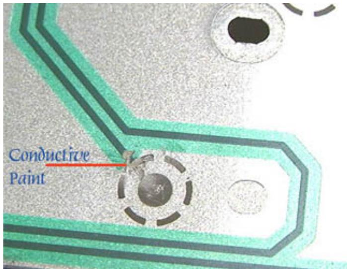
right, the unenhanced portrait of the same keypad after some conductive paint from a circuit trace repair pen was applied to the area between the insulated trace and the centre of the keypad.
