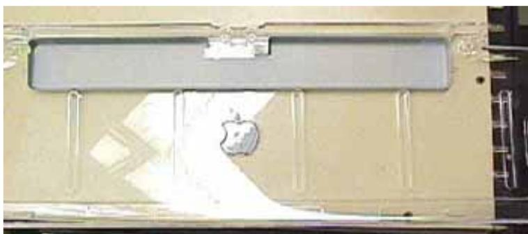
Place the PCB cover in the bottom shell as illustrated and prepare to set the keyboard in place. Before replacing the keyboard be sure to remove the three keys that cover the small Philips holding screws. These keys are the CAPS LOCK, semicolon (;) and numeric keypad number six (6) keys.
