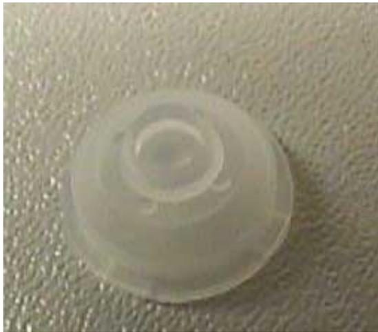
This is one key button. It is an elastic type of material which springs back into form after squishing. There are 109 of these, one per key on the keyboard. If you lose one, you lose the function of one key. These devices have a built-in plunger that - when pushed down by a key cap - pushes down on the top keyboard membrane and forces it to connect with the lower keyboard membrane, thus creating a connection which translates into a key press.
