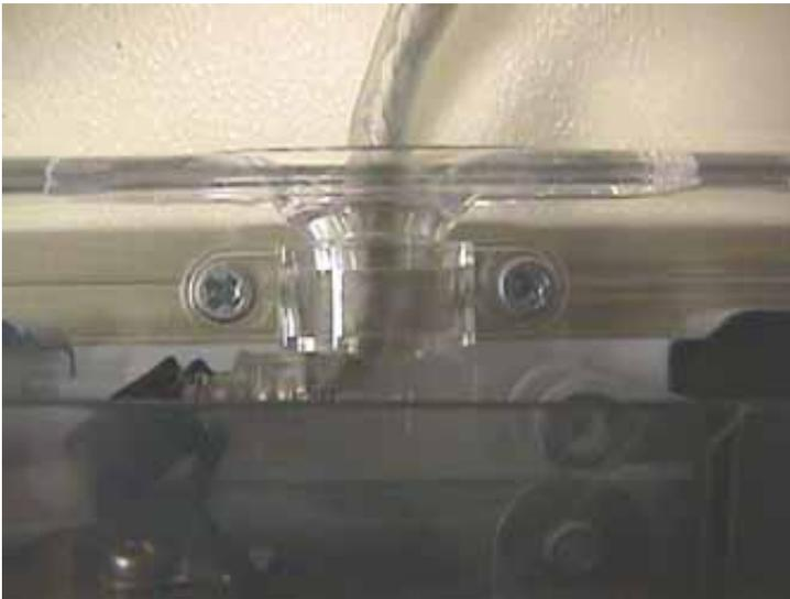
This is what the finished strain relief assembly looks like before the keyboard is placed correctly into the bottom shell. Note the plastic cover at the top of the keyboard that will interfere with the strain relief clip screws. This cover would prevent the use of a screwdriver to remove the strain relief clip before the keyboard is free of the bottom shell.
