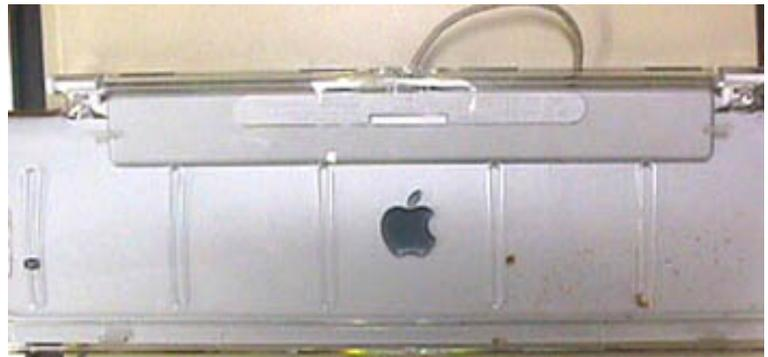
keyboard's centre. You can see in the image at right a few spots of cola that ended up at the bottom of the keyboard. Notice that near the bottom of the keyboard on the left and right ends there appear to be two more screws that grip the underside of the keyboard. If the keyboard is tilted sufficiently you can also find a third screw secluded by the lovely Apple logo in the centre of the shell.
