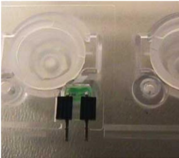
At left is a photo showing the LED in its place in the key button mold. The photo on the right shows the keyboard membrane at a point where one set of LED contacts can be seen. The two square pads near the centre of the image are what rest against the leads of the LED when the keyboard is properly assembled. The LEDs fit one way only into their respective places in the mold, so
