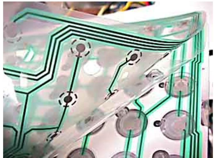
The tracks of green in this image are insulating coatings which ensure that the traces running between all the key pads will not come into electrical contact with each other through keystrokes or other external pressures. Even water or alcohol will not get under these coatings, which is good to know for cleaning purposes.
