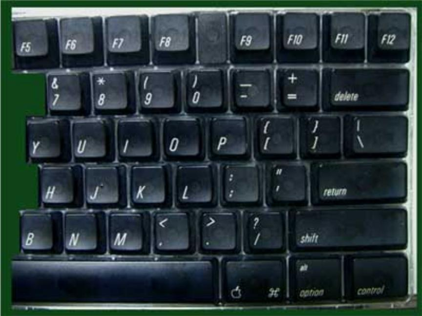
Here is what the centre portion of the keyboard should look like once all the key caps have been installed in the proper places.
