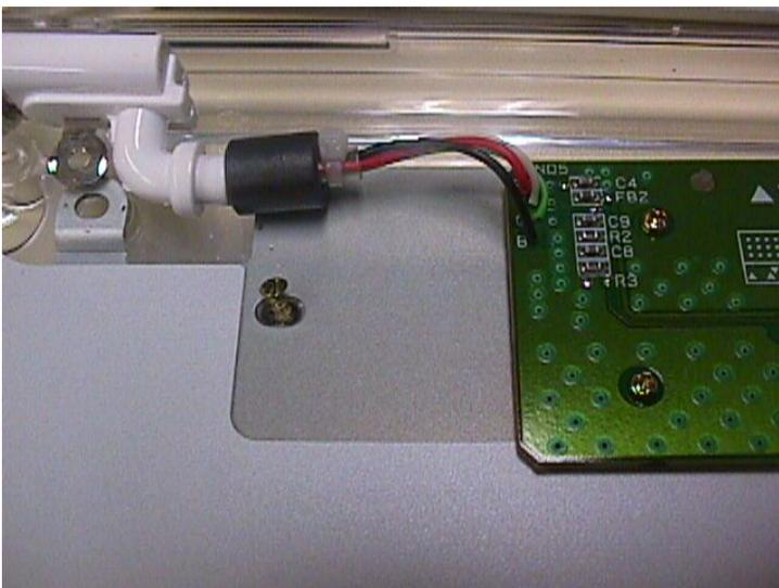
Note that pan head (or round head) Philips type screws are used to hold the PCB in place while the other screws found in the back plate have bevelled heads so they rest just below the surface of the back plate when installed properly. Remove all the pan head screws from the PCB.
