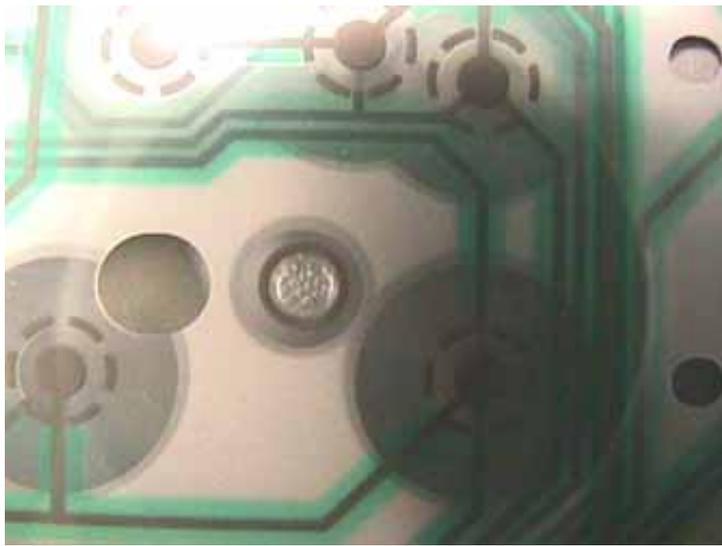
patterned circle to the right of centre where all three membrane layers have been fused together. The number one rule here is **DO NOT DISTURB!** If you tear the layers apart it will be difficult to perfectly align them in the future, and proper reassembly of the keyboard will be a long, trying process. While cleaning the membrane layers, try not to pry too hard against this fused spot and all will be well.
