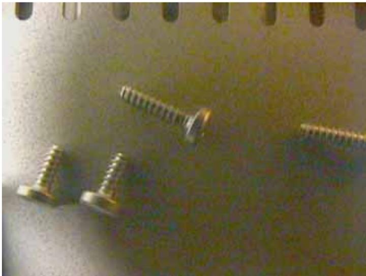
Notice that when these four screws are removed there are two pairs, each having a different length. This is important for proper reassembly later, so remember that the shorter ones are for the outer edges and the longer ones are used closer toward the
