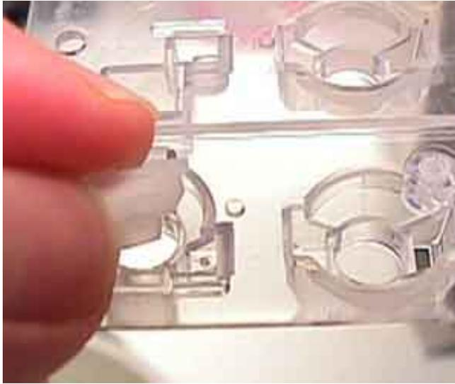
As if it wasn't obvious, the photo at left depicts the method of placing the key buttons into their mold - all one hundred eight of them! Place the mold on a flat surface and place all the key buttons in their spots. The photo at right shows what the small green LEDs look like. There are two such devices: one goes under the CAPS LOCK key, and the second goes under the NUM LOCK key at the top of the numeric keypad portion of the keyboard.
