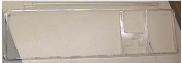
The photo at right shows the top keyboard shell and the photo at left is a close-up showing the snap together nature of the top and bottom shells. The
