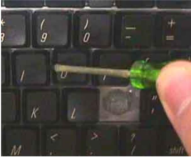
At this point you might as well remove all of the key caps as they must come off later in the process anyway. This will also make it easier to separate the top and bottom shells from each other when that time comes.
