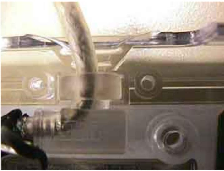
In order to fully separate the inner keyboard assembly from the bottom shell you must remove the keyboard cable strain relief. Once these two screws have been removed just pull the cable straight up off the bottom shell about an inch to release the strain relief mold from the bottom shell.
